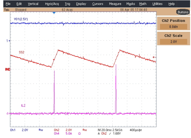
Figure 14 - 1.8V output shorted Ch1: Vo1, Ch2: SS2, Ch3: Inductor Current
