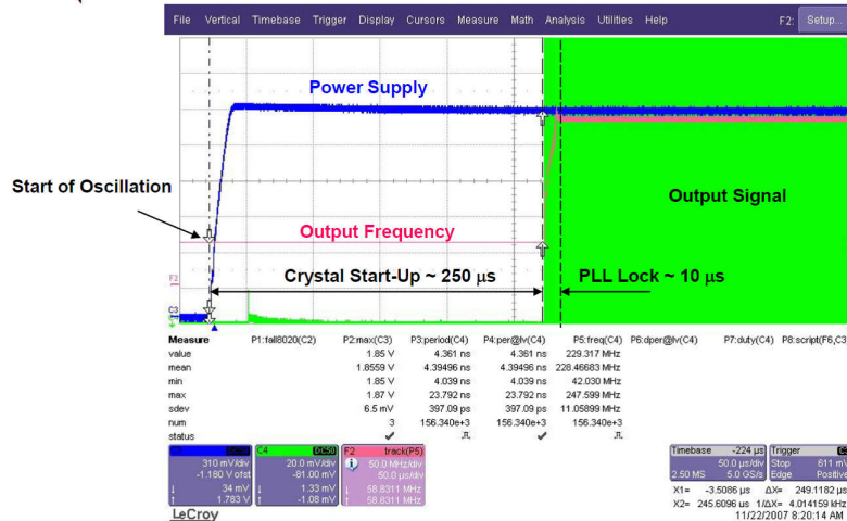
Figure 8-4. Crystal Oscillator Start-Up vs PLL Lock Time
