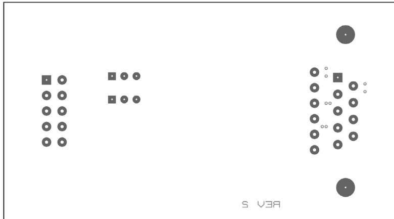
Figure 7e. Low EMI Demo Board Layout (DC1747A), Bottom Layer
