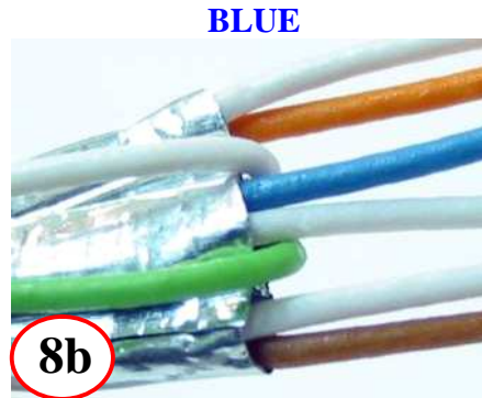
8b Split Grn pair around Blu pair, then fold back
