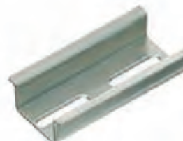
TS 35/15 mm according to EN 50022 (s = 1.5 mm)
