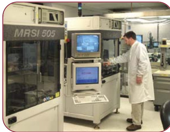
AUTOMATED EPOXY AND DIE PLACEMENT
