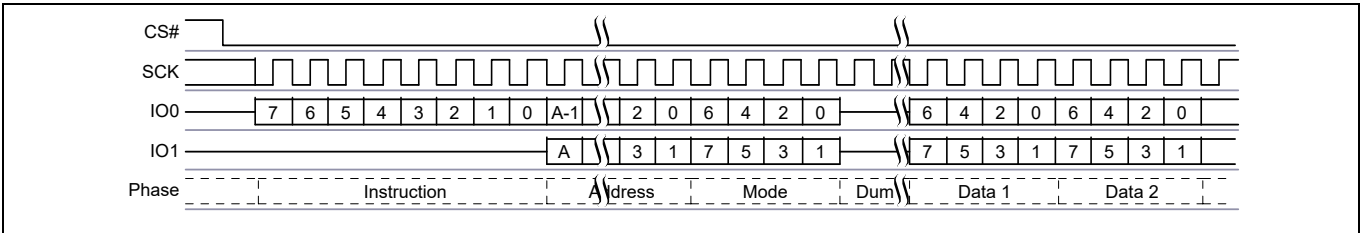
Figure 69 Dual I/O Read command sequence [32, 33]
