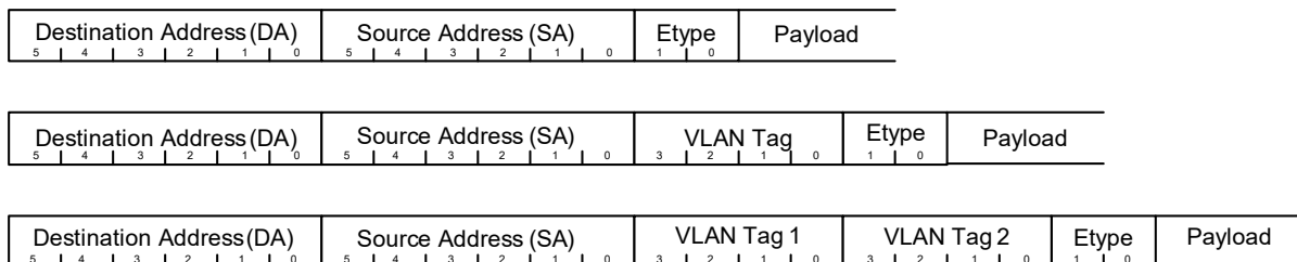
Figure 38 • Type II Ethernet Basic Frame Format
