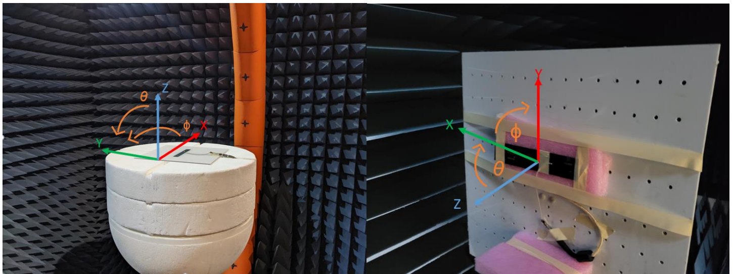
OTA Setup of the FXUB85.54.0150C in the SG24-L Satimo Test System For 600 MHz – 6 GHz Testing
