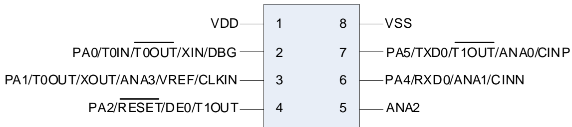
Figure 2. 8-Pin SOIC Package Diagram – Z8FS040xSB20EG
