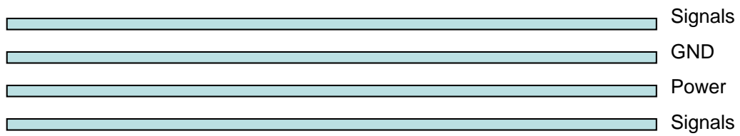
Figure 8: Typical 4-layer PCB construction
